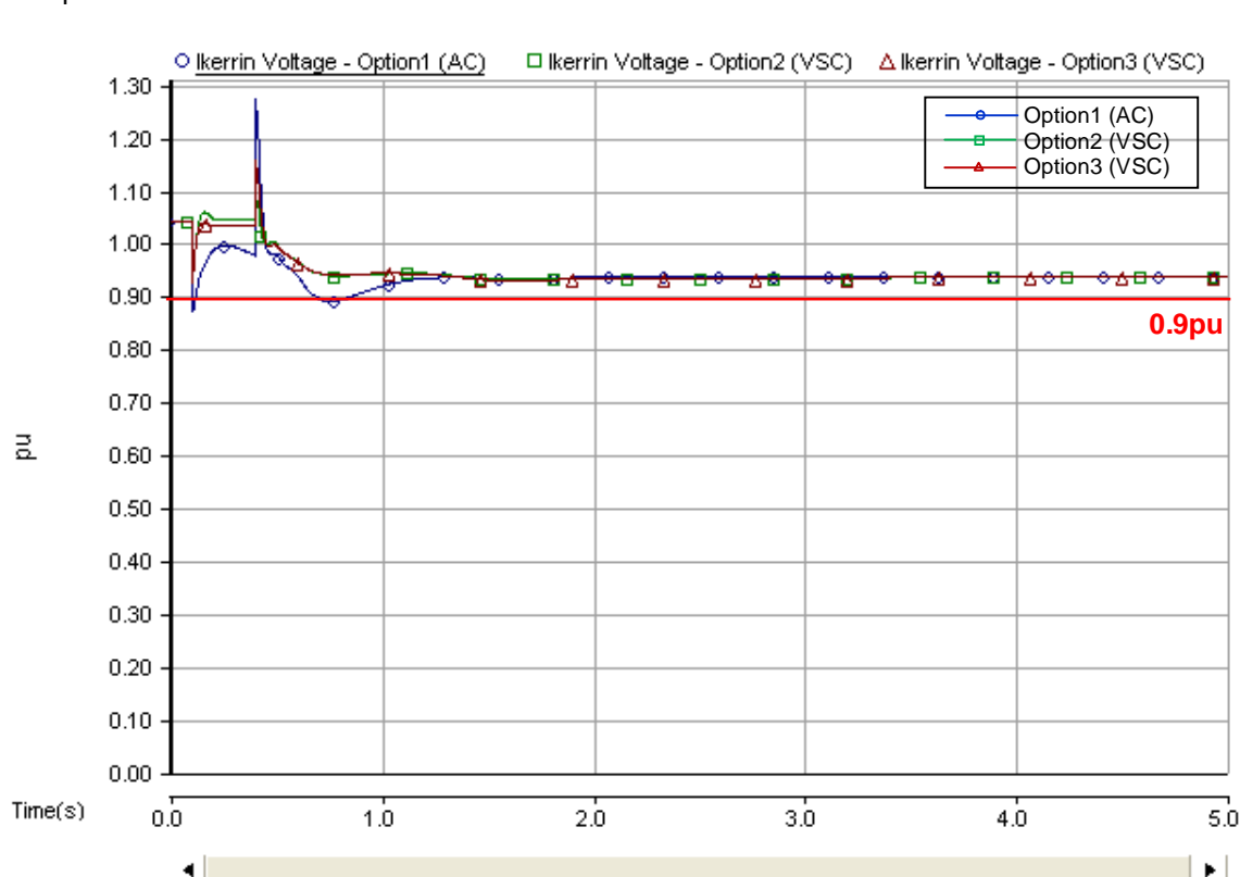
Figure 10.12: Ikerrin 110 kV bus voltage during the breaker failure at Cahir 110 kV terminal (Contingency 3_1_X in Table 10.1), with an SVC at Thurles.
