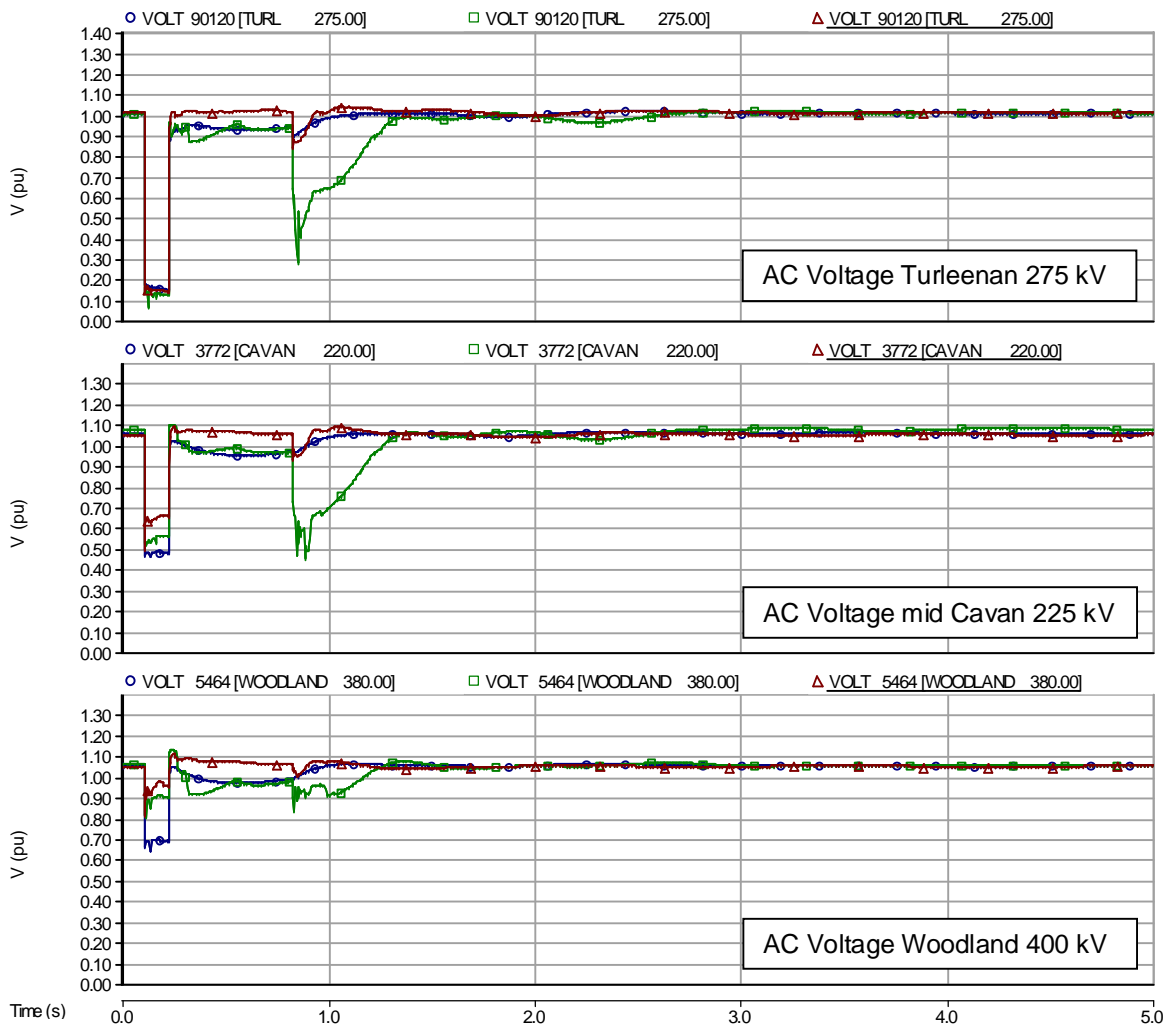
Figure 9.10. Fault at Tandragee followed by double circuit loss of Louth-Tandragee AC line and reclosing of lines 600 ms later. Comparison of terminal AC voltages in the AC, LCC and VSC options. (Blue – AC, Green-LCC, Red-VSC).
